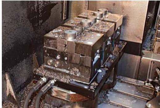
of the vice and one underneath the vice. The connection points have a 1/4" thread. These are hermetically plugged when not in use. The connecting points are used when the vice is positioned on the table. The vices are connected by means of rigid or flexible piping. These need to be heat proof to avoid burning chippings, etc. The underneath plug points do not need a thread connection and are installed with
